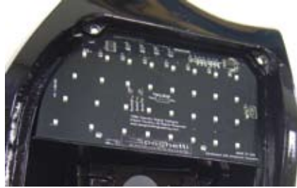
LED board in place.
