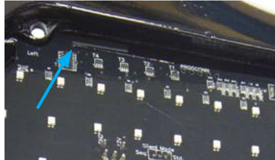
Arm portion sitting in gasket groove.
