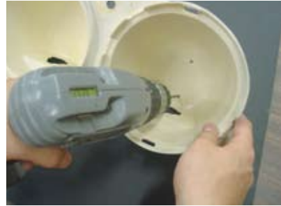
Drill marked holes.
