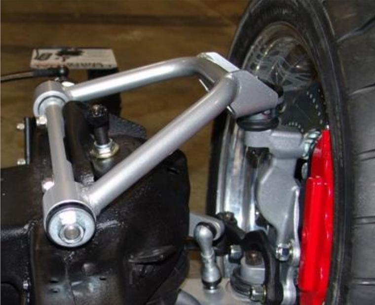
1. Fasten the upper arm to the frame using the factory hardware. Reinstall the current alignment shims, but **vehicle must be realigned.**
