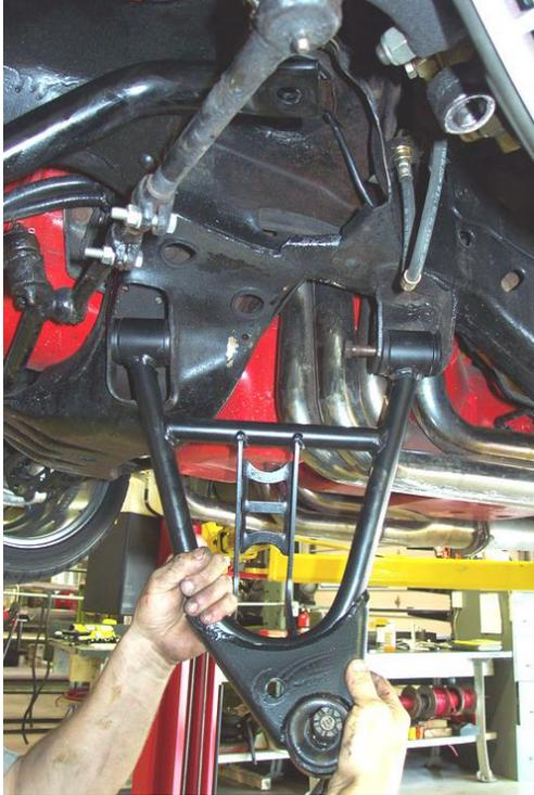
1. After removing the factory lower control arm, clean the bushing mounting surfaces on the frame to make sure they are fairly smooth.
