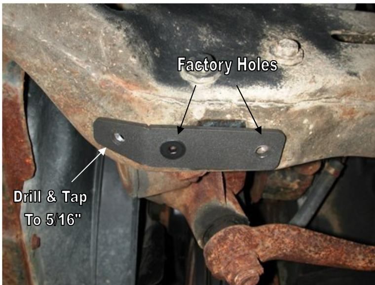
3. Bolt the frame plate to the frame using the factory sway bar holes. The front hole will use a 10mm x 30mm flat head Allen screw. The rear hole will use a standard 10mm x 30mm hex bolt.
