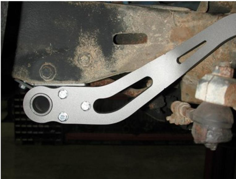
7. Bolt the sway bar arm to the bar using 3/8" x 1" Button head screws with flat washers and lock washers.
