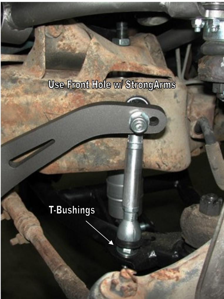
8. Fasten the 90 degree end of the PosiLink to the sway bar arm using a 10mm Nylok nut and flat washers
