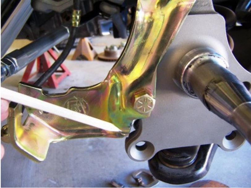
**Note:** If using a factory style stamped caliper bracket, the bracket may need to be trimmed. The dust shield may also need to be modified.
