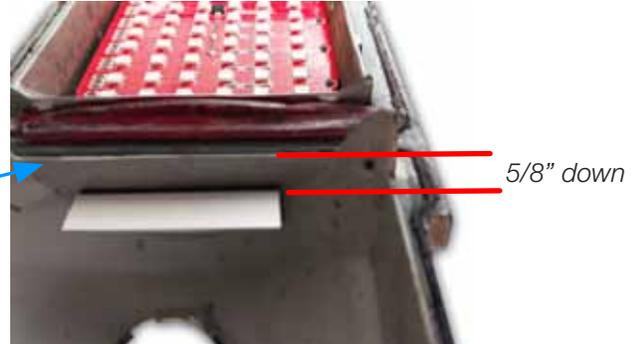
2. Attach an angle bracket with its face on the mark on the mark.
